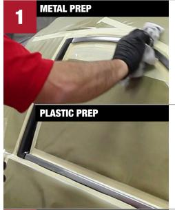
Clean with *SEM* Solve or XXX Universal Surface Cleaner. Wipe clean in one direction with dry, lint-free cloth. Sand with P400 grit and blow off. Re-clean with *SEM* Solve or XXX Universal Surface Cleaner. Wipe clean in one direction with dry, lint-free cloth.
