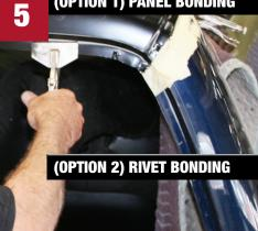
Clamp panel into place. Do not over clamp. Wipe away excess material.
