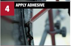
Apply 3/8" - 1/2" bead of **Dual-Mix**<sup>TM</sup> **Multi-Purpose Panel Adhesive** or apply 3/8" – 1/2" bead of **Dual-Mix Weld-Bond Adhesive** to both surfaces. Use enough material to completely fill the ioint when parts are clamped. Tool with a spreader or acid brush. Cover all exposed bare metal.
